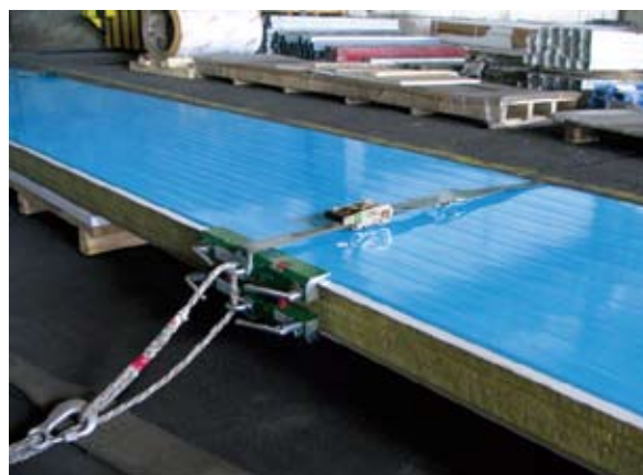
Pic. 5. Lifting assembly tool for Ruukki sandwich panels in vertical panel arrangement.
