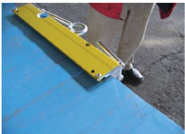
Pic. 6. Lifting assembly tool for Ruukki sandwich panels in vertical panel arrangement.
