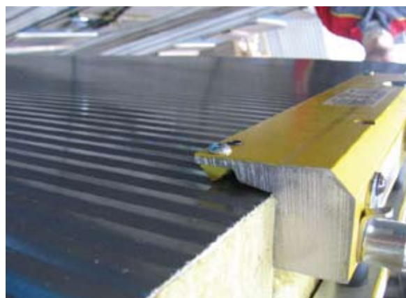
Pic. 7. Lifting assembly tool for Ruukki sandwich panels in vertical panel arrangement.
